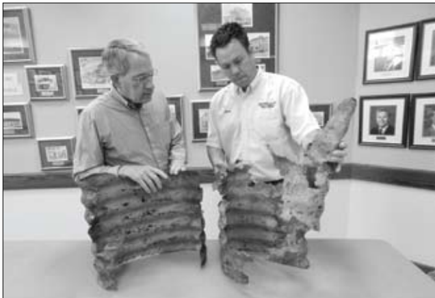
Drainage Utility Supervisor Dave Walker (right), shows City Manager Steve Thacker a piece of corrugated metal drain pipe that recently collapsed.
